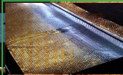
Reflective Insulation Blanket Applied to Roof, Slide-Out Floor, Entire Underbelly, Additional Wrap Around Holding Tanks
