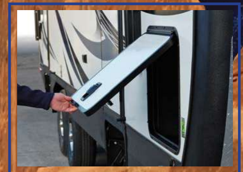
1" Thick Thermal Insulated Luggage Door Compartments
