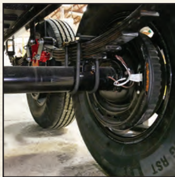
7K DEXTER EZ LUBE AXLES WITH NEVER-ADJUST BRAKES
