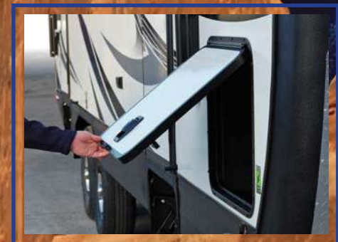
1" Thick Thermal Insulated Luggage Door Compartments
