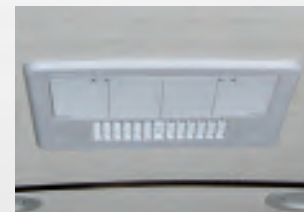
"Twice Cool" Dual Air Conditioning Duct System
