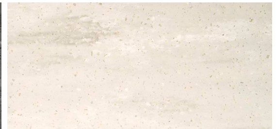
Neutral Aggregate Concrete
